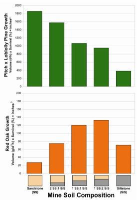
Figure 1. Pine and red oak production in topsoil substitutes consisting of different amounts of sandstone and siltstone. Tree growth is shown as an estimate of biomass volume x survival (ground line d<sup>2</sup>h x % survival/100) (Pine data from Torbert *et al.* 1990).
