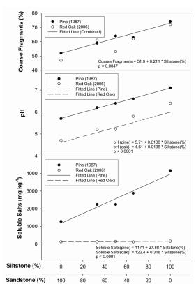
Figure 2. Coarse fragment content, pH, and soluble salt content for increasing amounts of siltstone versus sandstone used as a topsoil substitute for growing pitch x loblolly pines (1983-1987) (Torbert *et al.* 1990) followed by northern red oaks (2002-2006).
